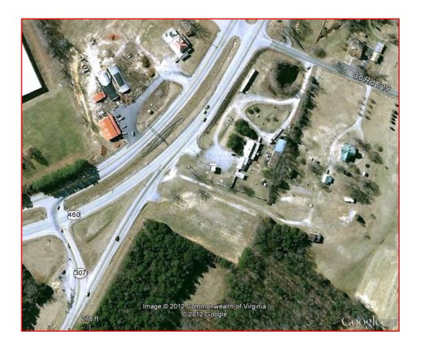
VDOT is also considering the possibility of realigning the entire intersection to bring all traffic to a T intersection to enter and leave Route 307. This would also move traffic away from Route 619 that is immediately after the exit from Rout 307 on Route 460.
